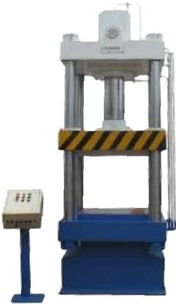
HYDRAULIC PRESS FOR HYDRO TESTING
